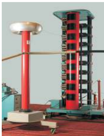
Impulse Test Set Up
